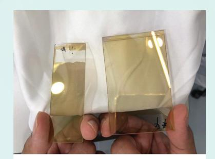
Left: Films deposited on glass substrate Right: Films deposited on acrylic substrate
